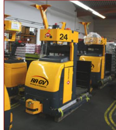
Above: the **RA-GV** fleet during customisation which will include a top-clamping platen for load stabilisation plus a second set of forks to deliver an empty pallet while simultaneously picking up a full one!
