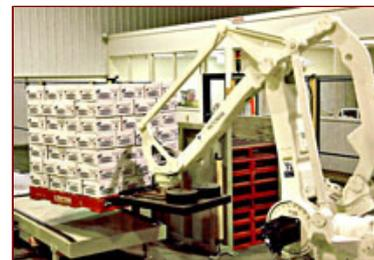
In a revolutionary design & layout, this one robot (with a reach of over three metres) picks varying products from SEVEN different machine lines onto SEVEN individual pallet-positions before turning into "forklift-mode" and lifting each full pallet onto an exit conveyor!
