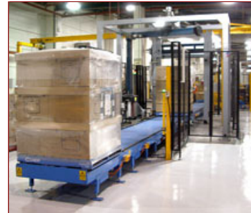
...At the other end, the RAGV can perform pick-up & delivery to warehouse racking or despatch departments. Note the neat presentation of wrapped pallet loads.
