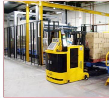
Above: The RAGV delivers a pallet-load to the ROBOPAC Helix HS30 wrapping station, where a top-sheet & full stretch-wrapping is applied...
