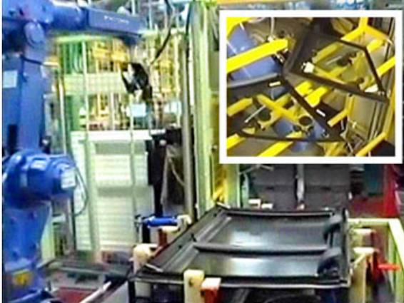
Above: Robo-gluing of roof-hatch. Inset: Pair of ready-glued side windows
