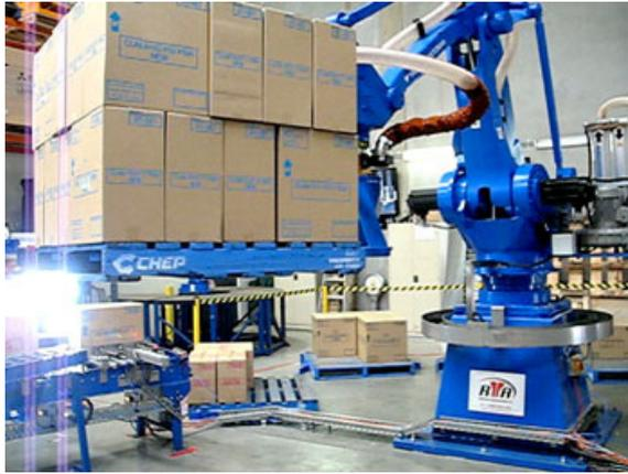
Above: Robot in robo-fork-lift mode and 3 of the 7 pallet positions beyond.
