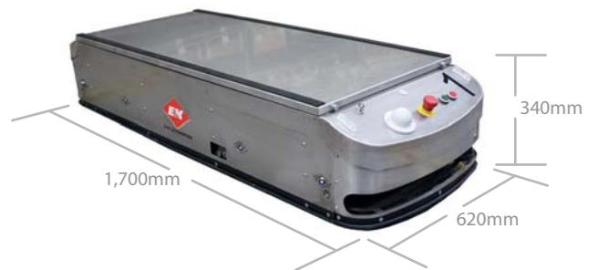
German-made, predominantly from high-grade stainless steel for hygiene and strength, the AGVs from E&K have a Super-flat profile to achieve a very low, sleek vehicle that's ideally suited to many hospital duties. With its integrated lifting gear, the vehicles deliver hospital trolleys, beds, containers and the like – up to 500 kg. The tried & tested design of the AGV is easy to maintain and delivers risk-free automated transport and handling.
