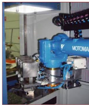
RA-designed camera above the Motoman HP50 robot with its multi-function gripper/dispensers.
