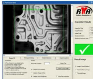
Vision software checks valve body position, clearance & insertion.
