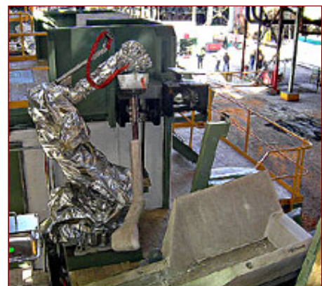
MOTOMAN HP200 robot (200kg payload - a big robot for 'The Big Australian') with foundry robot protection, heat-resistance jacket and end-of-arm fibre-stone paddle tool
