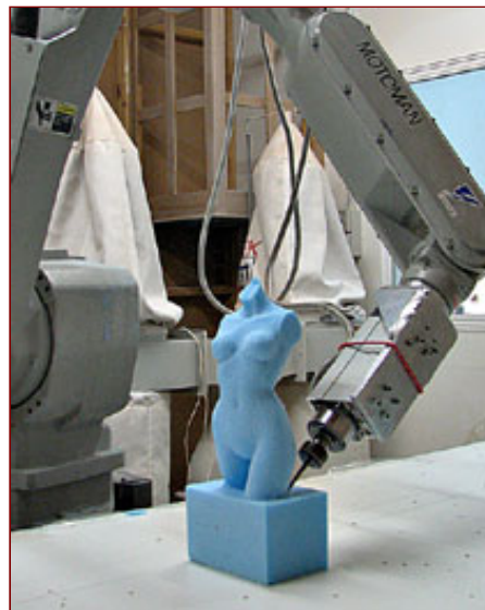
A styrofoam model sculpted by Tromes Design's MOTOMAN system
