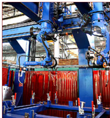
The MOTOMAN welding cell - largest gantry robot system in the Southern Hemisphere.
