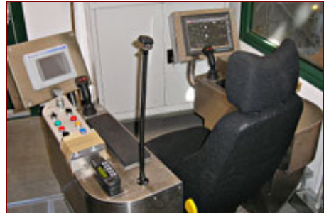
No, it's not Captain Kirk's command seat aboard the Starship Enterprise, but a purpose-built remote control station, with real-time robot control instruments.
