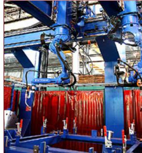
The MOTOMAN welding cell - largest gantry robot system in the Southern Hemisphere.
