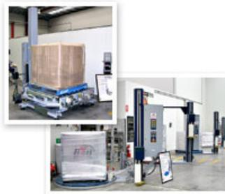
The ROTOPLAT 3000LD (top left) is a great value entry-level fully-automatic Stretch Wrapper with a rotating conveyor-plate. At right are examples from the rest of the range in semi-automatic ROTOPLAT systems
