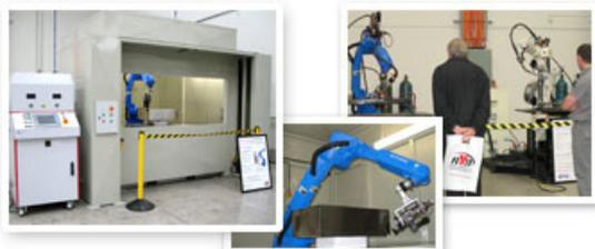
A robotic Laser Welding cell and MIG welding robots (at right) from MOTOMAN and OTC Daihen. All in action.
