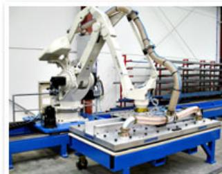
The first of 2 robotic systems on tracks of over 20 metres length. Here, the MOTOMAN EPL300 robot travels this length to serve 2.4m MDF wood panels to multiple label printing and CNC machining centres to create furniture components.
