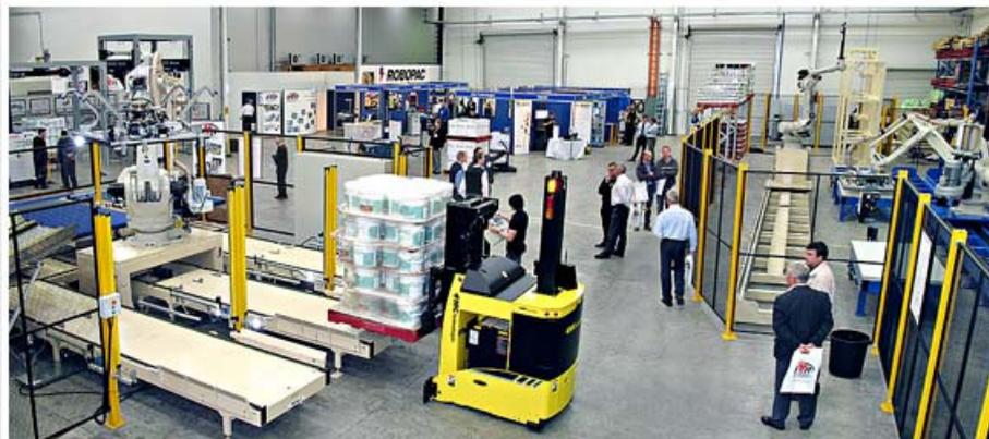
Above: an FMC Automatic Guided Vehicle (AGV) delivers a pallet load of empty pails to the robotic de-palletising system. Elsewhere, the AGV collects freshly palletised loads and delivers them to the "Genesis Futura" stretch wrappers (below) and then on to warehouse racking.
