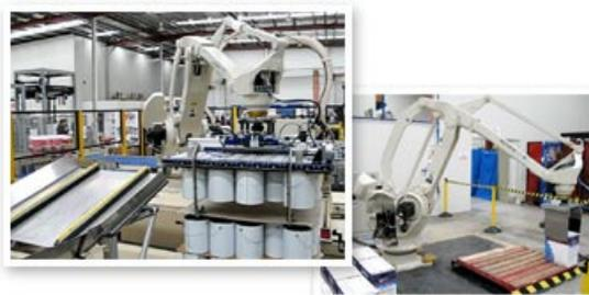
Left: MOTOMAN EPL300 Robotic De-palletising of empty paint cans -layer by layer - with vacuum gripper and second retracting gripper for slip-sheet removal. Handles multiple sizes of plastic & metal cans and serves 3 out-feed filling lines. Right: MOTOMAN EPL160 Robotic Palletising with pneumatic paddle gripper handling 20kg boxes of powdercoat product.
