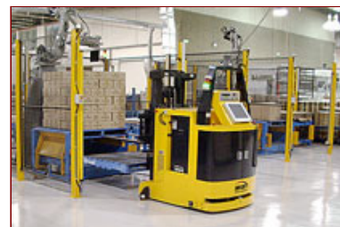
A new RAGV installation at AMCOR Sydney which also features robotic palletising & auto pallet wrapping.
