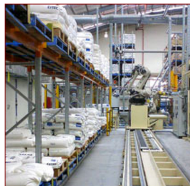
The Major Materials Fetching Robot glides down the pallet aisles collecting a list of ingredient powder sacks.
