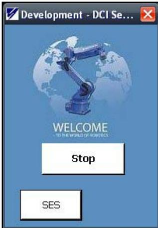
Visual Data Communication by Instruction (DCI) is an on-line communications protocol developed for Motoman® robots. The DCI Server software application allows the user to utilize this communications protocol to upload and download robot programs and variables.
