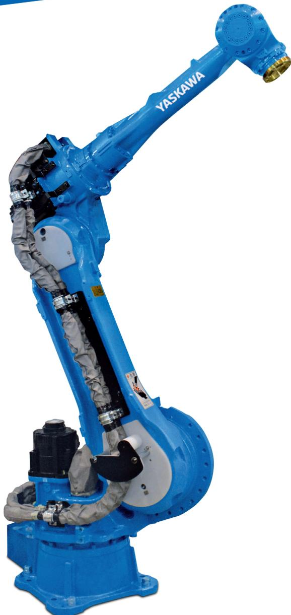
The MOTOMAN MS80W II is YASKAWA's answer to worldwide downsizing of spot-welding guns. This 80 kg spot-welding robot represents a further highlight of the company's range.
