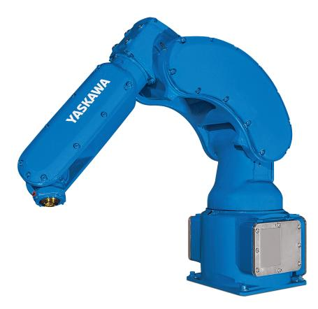
The compact MOTOMAN MPX1150 robot was developed especially for painting of small work pieces. It provides a payload of 5 kg for mounting multiple guns and small bells. Its high density layout saves space by reducing the size of the painting booth. The S/L axis is designed with no offset to enable installation of the manipulator closer to a work piece. The robot can be mounted on the floor, wall or ceiling and has three selectable access points for power cables.
