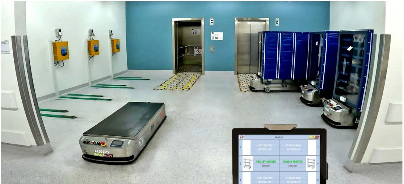
500 km (equal to 750,000 steps) of material movement per day using 14 dedicated lifts controlled by the MAXAGV Control System.
