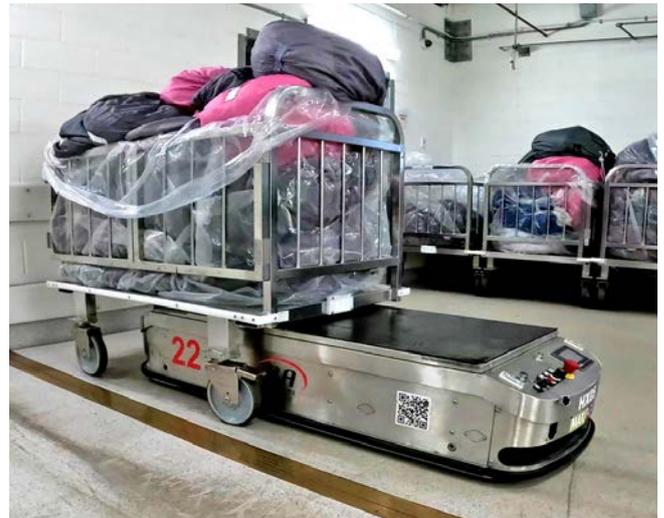
On-board RFID readers simplify and reduce the infrastructure required.
