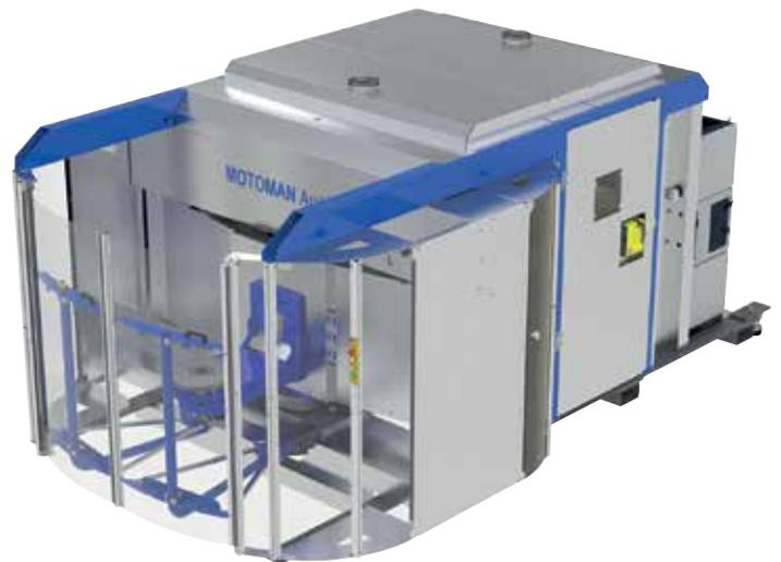
Each **ArcWorld CS** cell is prepared for TIG, MIG or MAG welding, depending on requirements. The positioner variants of different types and sizes ensure high work piece flexibility.
