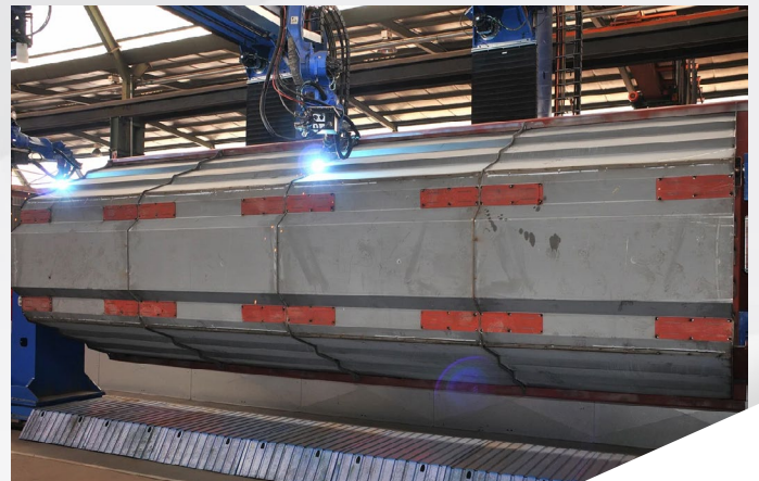
The entire gantry welding system is 24m long and the support pillars are more than 3m high
