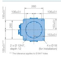
Mounting options: Floor, ceiling, wall, tilt\* IP Protection: IP67
